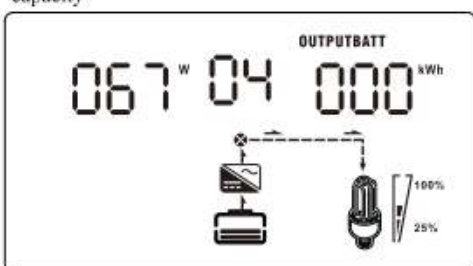
Page 06) Battery power percentage and remaining battery capacity (Note: The remaining battery capacity is only available when GRO, VLO and PAC lithium battery communication protocols are selected in Setting A16 and successfully connected to lithium batteries.)
